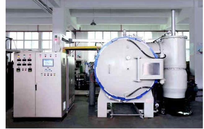
Electrical sintering furnace
