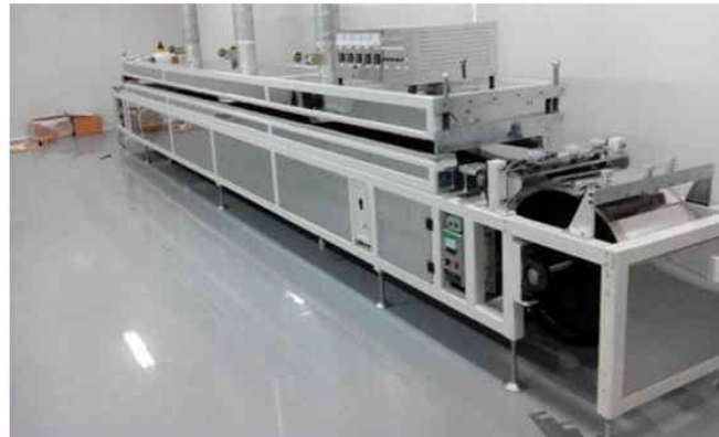
Tape casting machine
